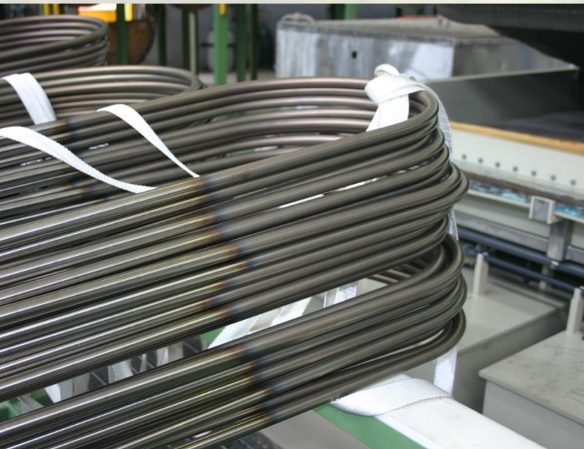
Bended tubes after annealing
