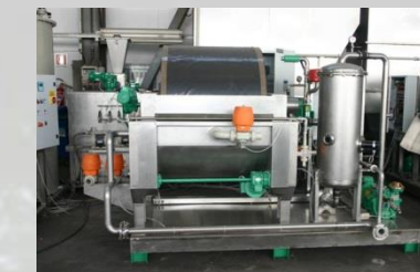
Sludge dehydrator with draining bags, with vacuum rotating filter, filter press.
