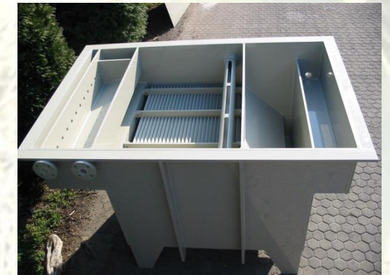
Pretreatment unit for breaking of the emulsions and lamella oil removal.
