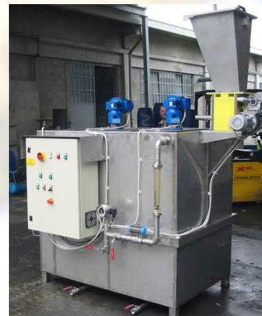
Unit for preparation and dosing of the polyelettrrolite.
